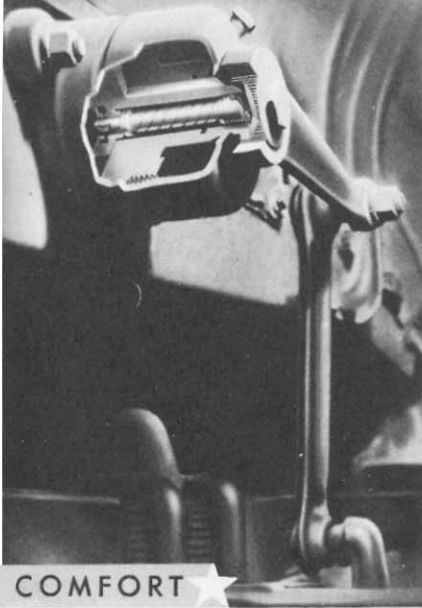
Automatic Ride Control, introduced by Studebaker in 1932, protects you against both the expected and the unexpected bump in the road without fumbling for a lever on the dash.
